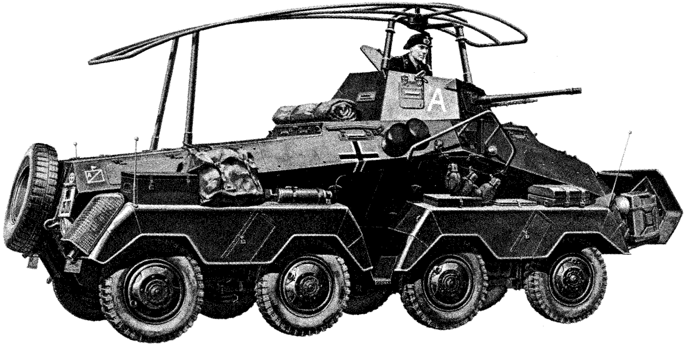
German Eight-Wheeled Heavy Armoured Car (Sdkfz-232)
