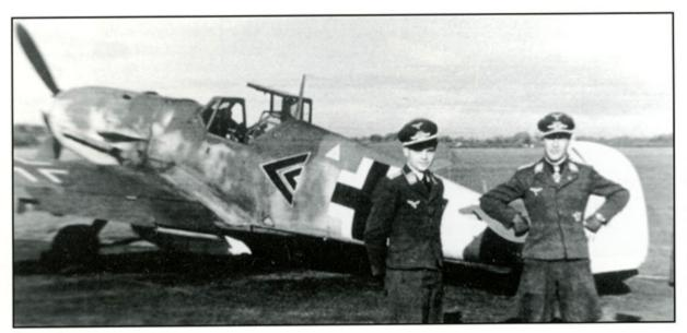
The tall antenna mast and missing DF loop are evident. The bright sun has lightened the Yellow band between the two men making it appear almost White.
