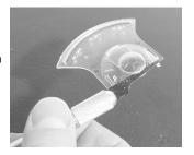
Cut out the bridge area from kit part 102. Remove at least 0.81" (21mm) wide, up to where the window begins.
