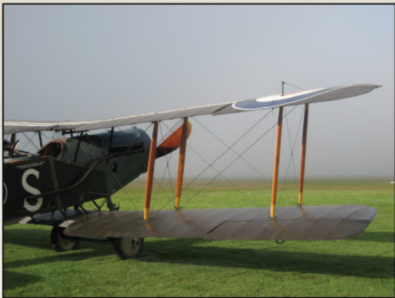
Starboard wings showing useful rigging details, note the late style extended exhaust.
