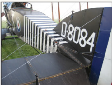
Tailplane showing the various control cables and RAF rigging wire details.
