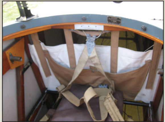
Rear of observer's cockpit showing the cloth screen and storage pockets, usually used for extra Lewis Gun magazines. Note the post WW1 four point safety harness.
