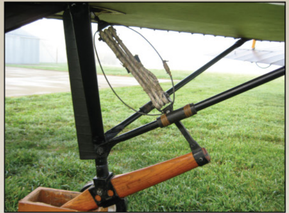
Tail skid showing bungee cord and retaining wire details.
