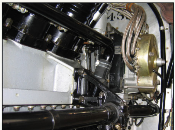
View of the left magneto showing plug leads and colouring details.
