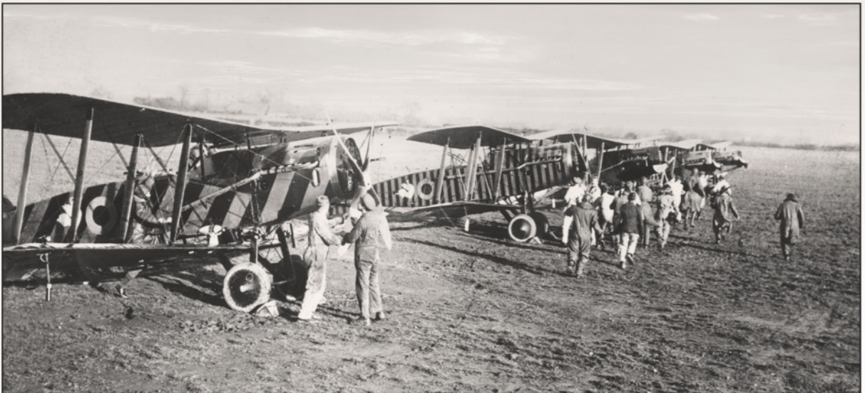
A line up of night fighters displaying a variety of interesting colour schemes. The colours are again unknown but could have been yellow with black or red stripes. Note the wing mounted generator and Holt landing flares on the aircraft in the foreground.
