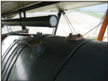
Aldis sight, front fuel tank filler cap and Vickers Gun magazine loading hatch details.
