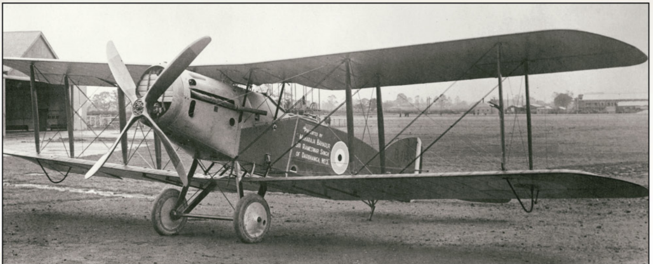
Note the early style undercarriage V struts and small magneto access hole in the engine cowling of this presentation aircraft. For additional colour schemes, high resolution photos and ideas for modifying your model please visit www.wingnutwings.com .
