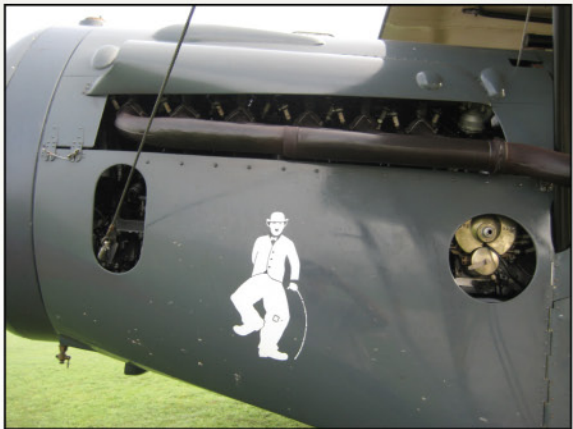
Engine cowl detail from D8084. Note the drift cable exiting the engine bay through the air scoop hole (the actual scoop has been removed). Period photos show that these cowling air scoops were often removed in service.
