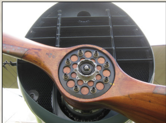
Note the propeller boss and open radiator shutter details.
