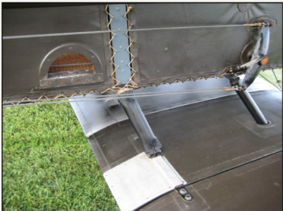
Starboard lower wing center section showing reinforced metal steps and elevator controls. Also note the lacing between the fabric and metal fuselage sections.
