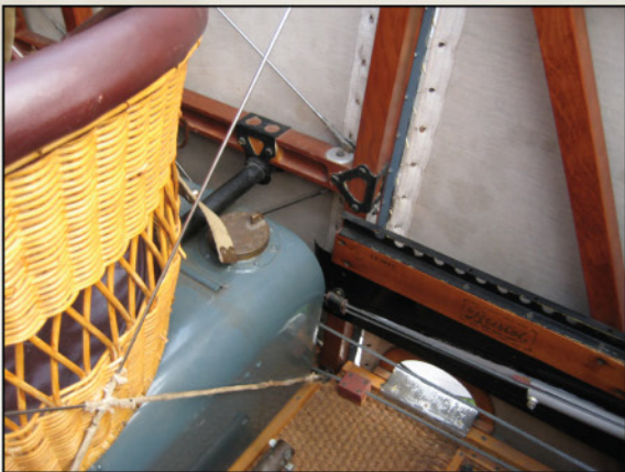
Rear of pilot's seat showing the rear fuel tank and fuselage foot step details.
