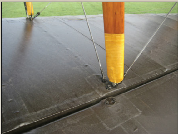
Port lower wing outer struts showing yellow reinforcing tape.
