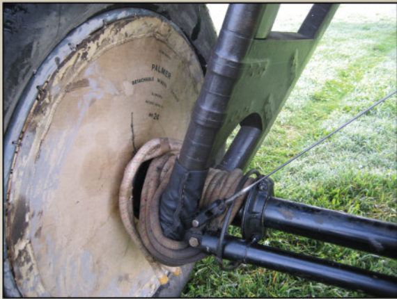
Right side wheel detail showing later style re-inforced undercarriage struts, note the bungee shock cord and axle retaining wire.
