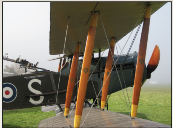
Starboard wings showing useful rigging details, note the late style extended exhaust.
