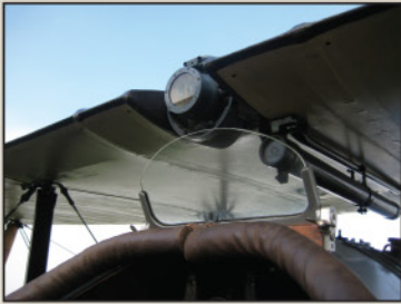
Windscreen, Aldis sight and compass details. Note the leather cockpit padding join at the centre.
