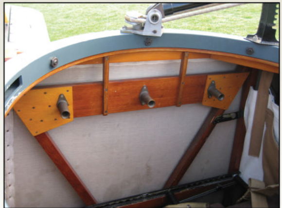
Right side of observer's cockpit showing mounts for spare Lewis Gun magazines. Note the interior colour of the fuselage linen.
