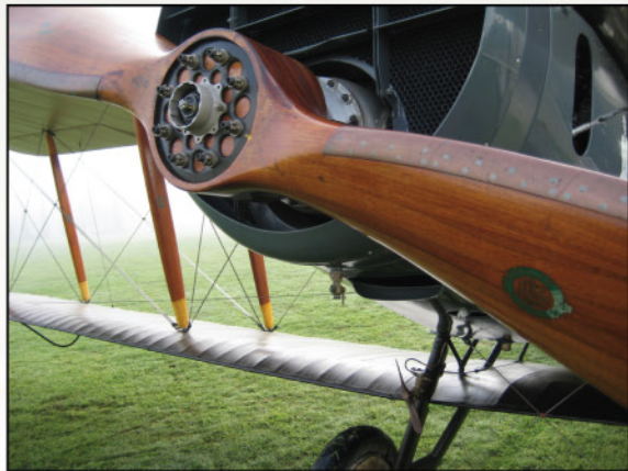
Interesting photo showing cowling, radiator and propeller details. Note the metal on the leading edge of the propeller and the carburettor drain pipe tap at the bottom of the radiator, details not always present in period photographs.
