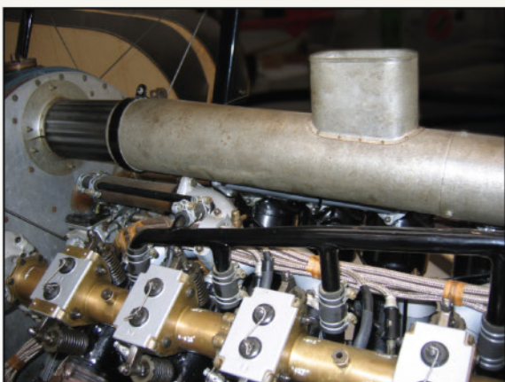
Vickers gun blast tube, note the gas exhaust outlet on top.
