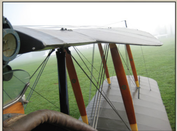
A pilot's eye view along the starboard wing showing strut decals and aileron control cable details.
