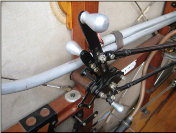
Left side of pilot's cockpit showing the throttle, mixture and spark advance control levers. Note the modern plastic tubing.
