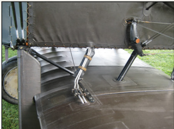
Port lower wing joint showing the pipes running out to the pitot tube.
