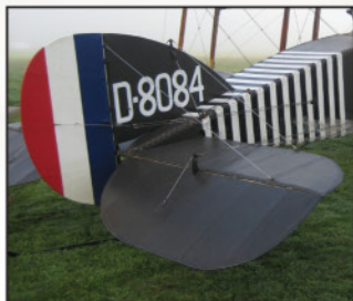
Tailplane showing the various control cables and RAF rigging wire details.
