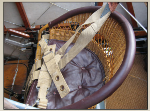
Pilot's wicker seat details, note the post WW1 Sutton four point safety harness.
