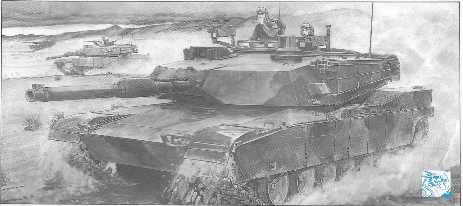
The M1A2 is basically a modified version of the battle-tested M1A1 main battle tank. Among the significant features of the M1A2 are: compartmented fuel and ammunition, automatic fire detection/suppression, thermal imaging/night sight, day/night fire on the move capability, NBC system, digital electronic control unit and others.
