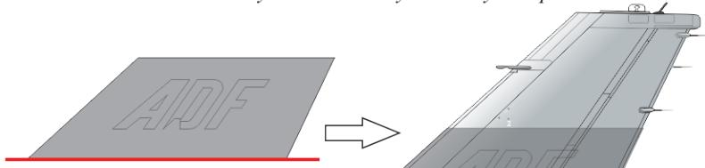
For the variant C: remove the top layer and cover yellow areas by a tape for painting. Use the mask contour as key.
