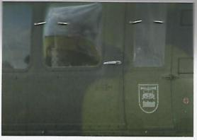
The above photo shows a bulged cabin window on a German Army UH-1D at the R.Neth.AF Show at Twenthe in 2003. The installation is typical - either the front or rear cabin door window can be replaced with a bulged version. This aircraft was unusual in that the starboard cabin door had a bulged window (illustrated), but the port door did not. Apparently, someone had broken it shortly before the aircraft left for the show...
