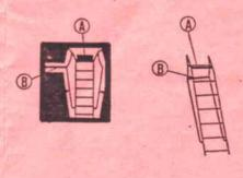
We advise you, for folding up the metal without any problem to lean you on the edge of a plastic plate and to use a pliers for all the manipulations you will have to do, the pieces being rather fragile when they are cutted off form their frame. For assembling, it is necessary to use a cyanoacrylate glue.
