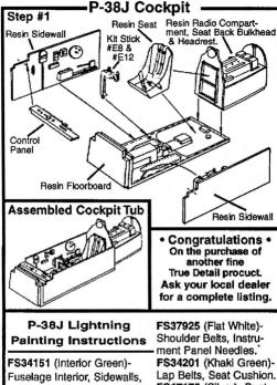
FS17178 (Silver)- Seat Floorboard, Seat. Belt Buckles, Rudder & FS37038 (Flat Black)- Instru-Pedals. ment Panel, Gunsight, Radio FS30117 (Leather Box, Battery Box, Trim Wheel, Brown)- Headrest Cush-Throttle Quadrant, Instrument ion & Chafing Pads on Panel, Various Equipment Lap Belts. FS34092 (Dark Green)-Panels, Oxygen Regulator, Oxygen Hose. Control Stick & Grip.
