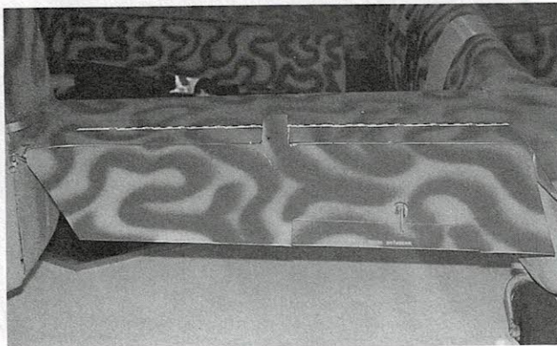
At left is a photograph of the left elevator on the horizontal tail. The trim tab and its actuator can be seen in this view. At right is the left vertical tail. The marker in both pictures is a ruler which has been painted with black and white one-inch segments to provide a reference for size.
