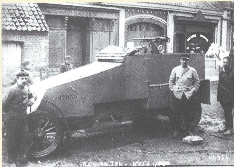
Illustration 5. Another 17935 Renault armoured car on the streets of an unknown town, again without the MG shield.
