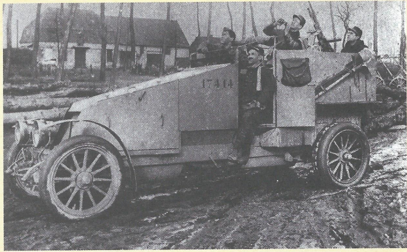
Illustration 4. This classic photograph, taken from the press of the time, was taken in March 1915. The group to which car 17414 belongs is not known. Note the MG shield removed to fire against the aeroplanes.
