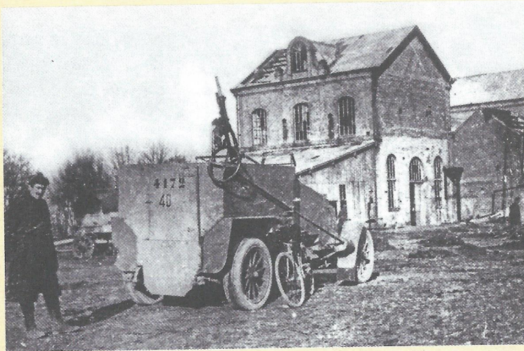
Illustration 3. The special device visible on the right side of this armoured Renault is the first known example of an inverter on a French armoured car. Organized in a perfectly inconvenient way, it was not to be adopted. The other interesting aspect of this photograph is to show markings on the rear of the car, a detail rarely observed. The machine gun is in position for firing against aircraft. Winter 1915-1916.
