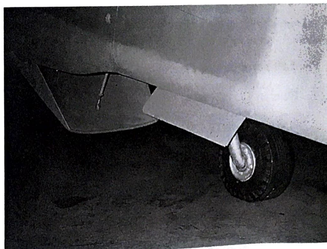
Details of the hot air exit ramp and the tail wheel can be seen here. (Detail & Scale photo by Bert Kinzey)
