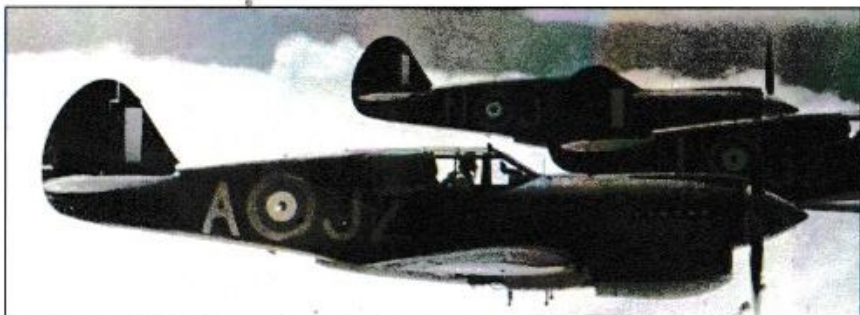
A photo of P-40E NZ3038 based at Ohakea, 1943. Like NZ3034 the individual aircraft code letter is behind the roundel on both sides of the fuselage. (RNZAF)
