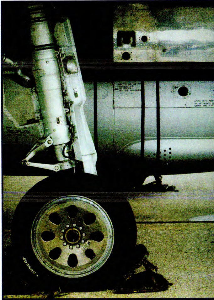
F.2A Starboard Main Undercarriage Leg and Wheel [note 'dished' style of hub on F.2A] - Photo Copyright David J. Parkins
