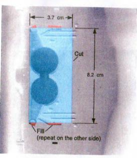
Remove the shaded area and fill as shown
