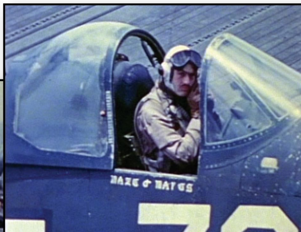
Two stills of "Maze & Hayes". We can only assume the aircraft was named for Maj. Maze and another VMF-511 lost on operations. Note the Gloss Sea Blue paint worn off (?) of the hand hold below the windscreen. No white tip on the prop hub, and the small aircraft numbers were only carried on the upper cowl lip and the forward main gear doors, unlike "My Nel III".
