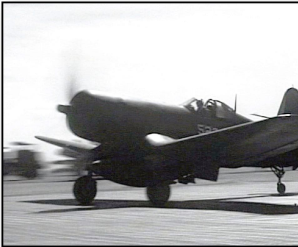
Three frames from a motion picture that show the unusual markings carried by 57522. Note the Neutral Gray 43 (?) 165 gallon Lockheed drop tank, the lack of a tail hook in the hook well, and the small aerodynamic fairing aft of the tail wheel.
