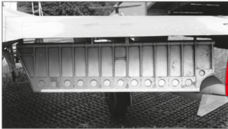
View of the unique Flap of the Hunter MK.50 / Mk. 50a and TMk. 60. The cut-out became necessary when the new 150 GAL FLUNT were introduced.
