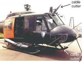
NOTE unusual arrangement for flotation gear on the aircraft above - it seems to be supported at the rear by a yellow and black bracket. This would normally only happen to allow manoeuvring wheels to be fitted to the rear of the skids.
