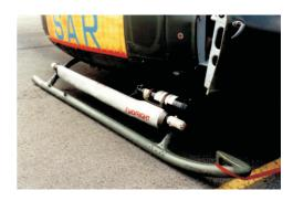
Notice how the flotation bags are attached at the front and rear.
