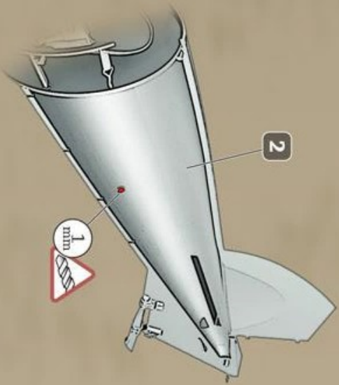
4 Drill hole for OAW lifting handle F17
