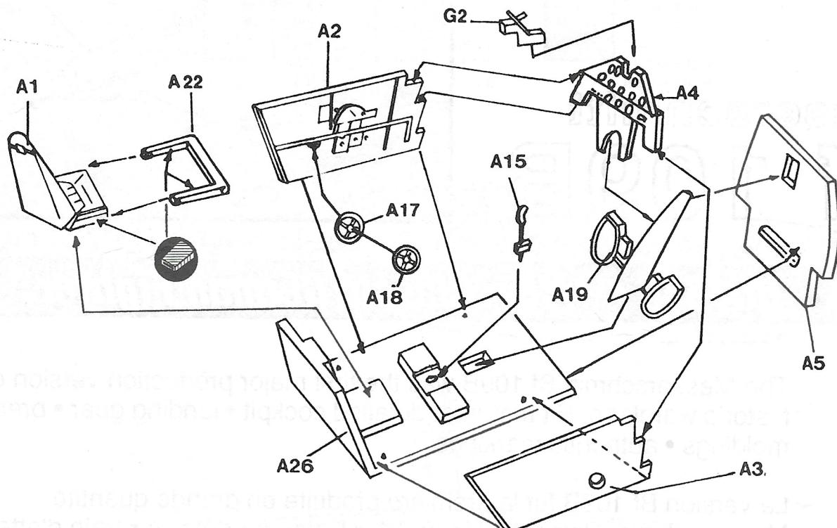
**2****Fuselage Assembly / Assemblage du Fuselage**
