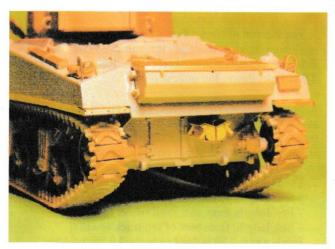
This picture shows the location of the 'Firefly' bin and its etched lid. These were often to be found on other vehicles, and in different locations. Also shown are the rear mud guard mounting strips, smoke emitter boxes and rear light
