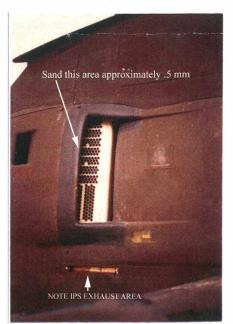
Sand the inside of the opening flat. If you can save the driveshaft inside the opening, great. If not, this can be replicated with round styrene rod after drilling a hole in the IPS inner face.
