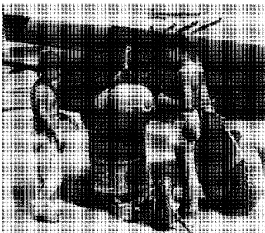
Armorsers load a 500-pound bomb on the right pylon of a Thunderbolt. A 55-gallon drum is being used on a standard bomb dolly for this purpose. A bomb dolly like this one can be found in ProModeler kit number 5930, WW-II GROUND EQUIPMENT. (U. S. Air Force Museum)
